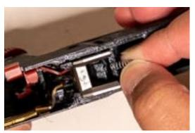
Insert the slide lock spring into the slot.
