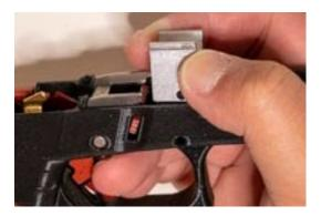
Insert the front rail block downwards into the frame.
