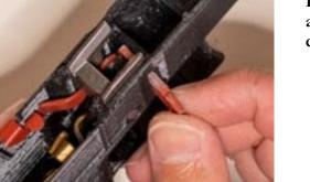
Insert the slide lock at an upwards angle and use the slide lock to press down on the slide lock spring.
