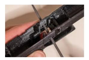
Ideally, the holes should not have any left over debris and filament stuck in them.
