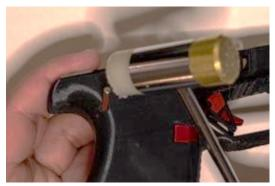
Install the trigger housing pin into the frame to secure the rail and housing.
